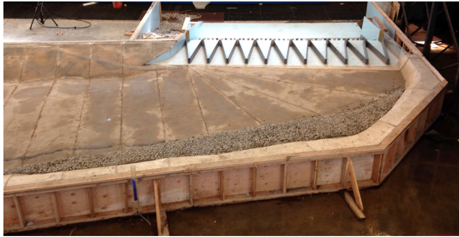
Fig. 29. Overhead view spillway model study with a significant approach flow angle
